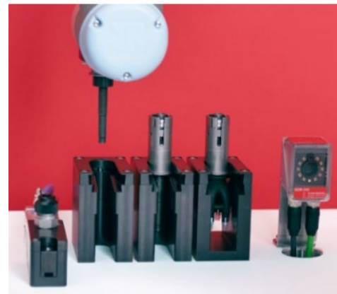
From left-to-right: external supply, 3x tool station, encoder
