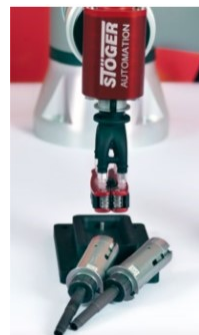
From left-to-right: external supply, 3x tool station, encoder
