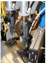
Above left: Close-up of SD-185 Screwdriver tooling on a horizontally mounted driver.
