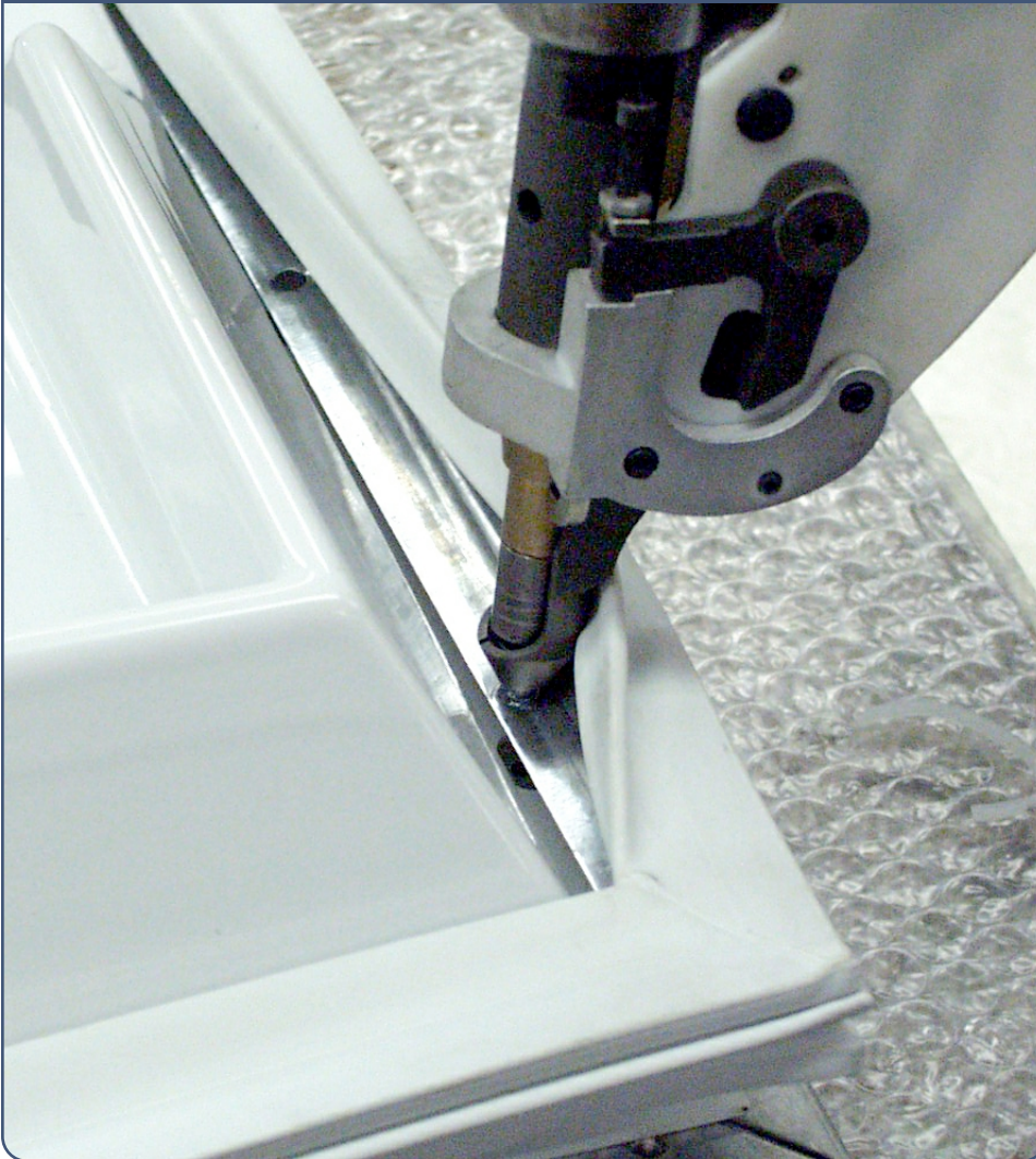
Photo shows chuck jaws transferring a screw from delivery tube to drive position
