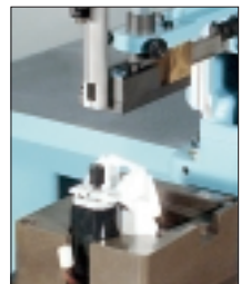
Model AP-120 Part Placer tooled to feed, place, and press a worm pinion onto a D.C. motor shaft.
