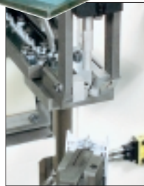
Model AP-111 Part Placer tooled to feed, place, and press an off-set cam onto a D.C. motor shaft.
