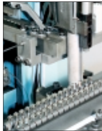
Model AP-111 Part Placer tooled to feed and place terminal springs onto a buss bar.
