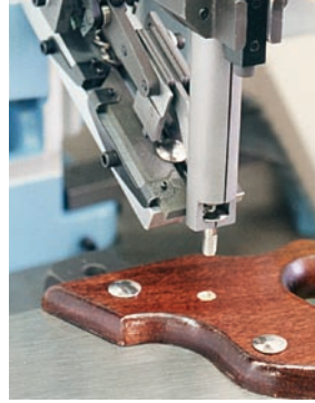
Model AP-107 Part Placer with 175 pounds (778 N) pressing force, tooled to feed, place, and press special truss headed fasteners into saw handles. The square shank section below the head is pressed into saw handles to keep the fastener from rotating.
