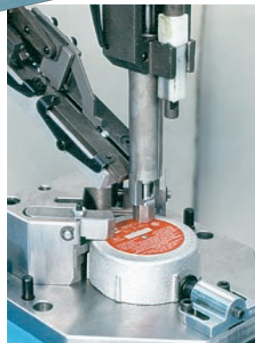
Model AP-110 Part Placer tooled to feed, place, and press a round head drive screw to retain a nameplate on a casting.
