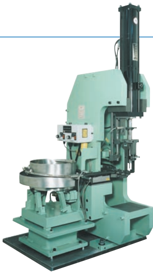
Model AO-712 Placer/Press with Bowl Feeder, Inline Track and Cross-Shuttle Escapement. Tooled to press a slug into a lock body.
